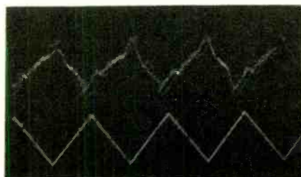
Fig. 4a—Sawtooth pattern of violin bowed carefully. b—Composite photo of violin waveforms, compared with triangular output of H-P low-frequency function generator 202A.
