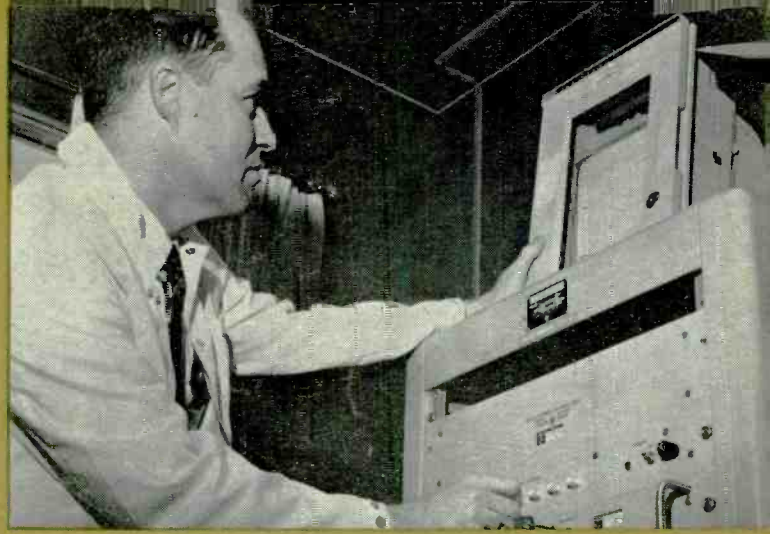
CALIBRATION OF PRECISION MEASURING EQUIPMENT used in the missile program is performed in Mr. Welch's section of the Laboratory. He is shown making an adjustment on the oscillator which is used as a frequency standard in this important task.
