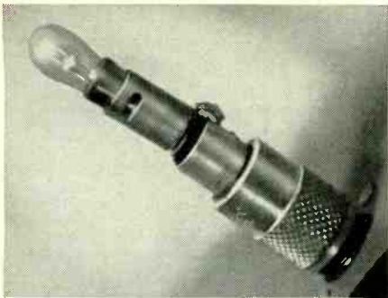
Fig. 5—Pilot light socket, pilot light and antenna connector used for dummy antenna.
