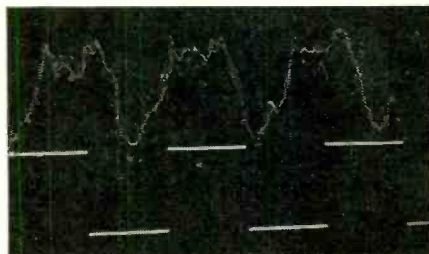
Fig. 5—Attempt to bow the violin with medium pressure and slow stroke to obtain a square wave. Square wave from signal generator is shown below, for comparison.
