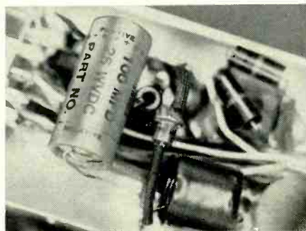
750-ma top-hat type silicon rectifier used to replace rectifier for keying relay voltage.
