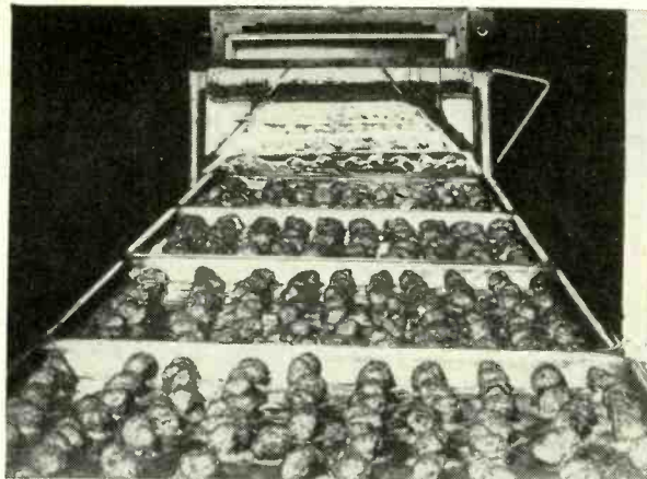
These trays of meat balls were cooked by quartz infrared heat lamps.
